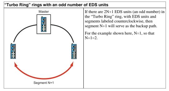
Determining the Redundant Path of a "Turbo Ring V2" Ring
